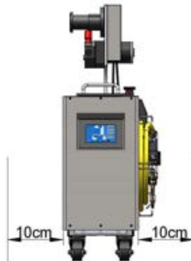
Figure 2.2.2 Placement space requirements
