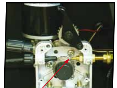
(8) Feed wire over the drive roller into the outlet guide tube, Push the wire through approx 150mm.
