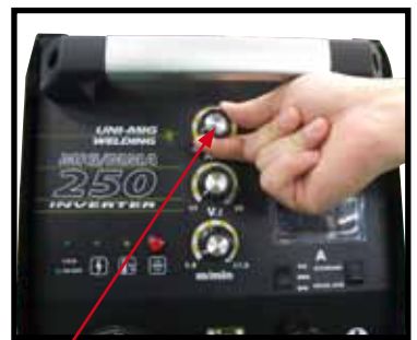
(7) Set the welding current using the amperage control dial
