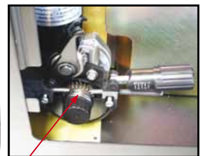
(9) Install a U groove drive roller of the correct size for the diameter wire being used.
