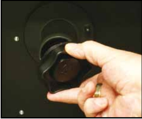
(1) Remove the spool retaining nut.
