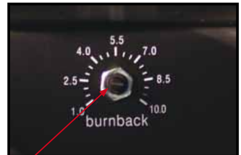
(17) Adjust the burn back control to prevent the wire sticking in the weld pool. Burn back control is located above the wire feed motor
