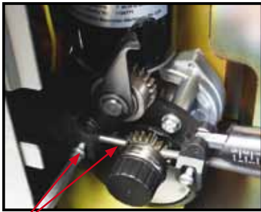
(10) Loosen the inlet guide tube retaining screw.
