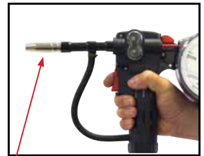
(15) Fit the gas nozzle ready for welding.
