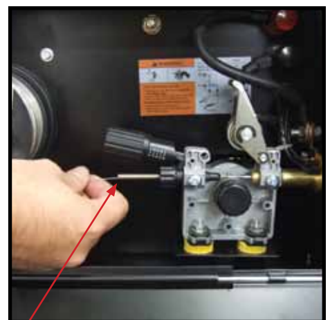
(7) Place wire onto spool holder - (spool retaining nut is left hand thread ) Feed the wire through the inlet guide tube on to the drive roller.
