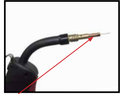
(13) Fit the correct size contact tip over the wire and fasten tightly into the tip holder.
