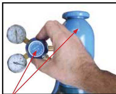
(16) Carefully open the valve of the gas cylinder, set the flow to 8-12 l/min
