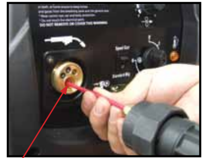
(12) Carefully feed the PA liner into the inlet guide tube hole of the torch euro receptacle
