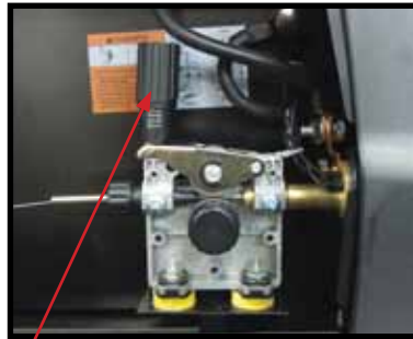
(10) Apply a medium amount of pressure to the drive roller
