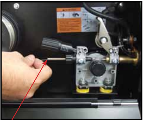
(7) Place wire onto spool holder - (spool retaining nut is left hand thread ) Feed the wire through the inlet guide tube on to the drive roller.
