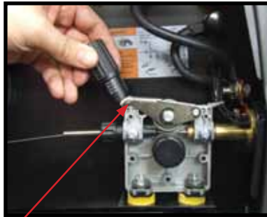
(9) Close down the top roller bracket and clip the pressure arm into place.
