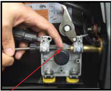
(8) Feed wire over the drive roller into the outlet guide tube, Push the wire through approx 150mm. Use a Knurled Drive Roller of the correct size
