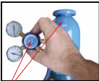
(15) Carefully open the valve of the gas cylinder, set the flow to 10 l/min
