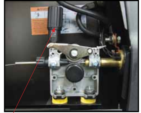
(6) Lock down the top pressure roller and apply a medium amount of pressure using the tension adjustment knob
