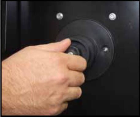
(1) Remove the spool retaining nut.
