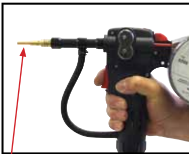
(13) Fit the contact tip over the wire and screw it into the tip holder, nip it up tight.
