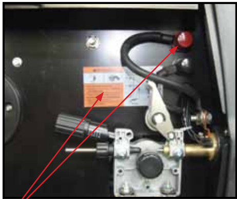
(6) Connect weld power lead to GAS ⊕ as show in picture inside machine
