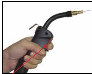
(12) Press and hold the inch wire button to feed the wire down the torch cable through to the torch head.
