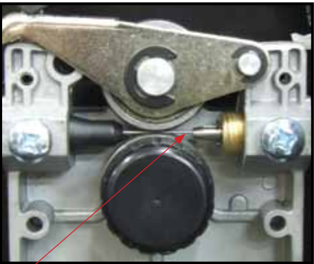
(7) Check that the wire passes through the centre of the outlet guide tube without touching the sides.
