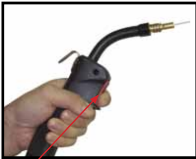
(12) Press and hold the trigger on the mig torch until wire is visible at the tip holder.
