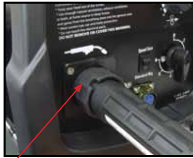
(14) Tighten and secure the torch euro connector to the machine euro receptacle
