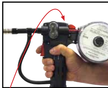
(14) Adjust the drive roll pressure if required by using the adjusting screw at the top of the torch.
