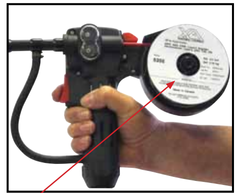
(9) Place a spool of wire onto the Spool holder.
