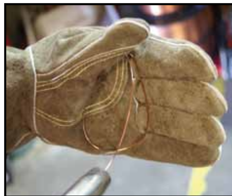
(8) A simple check for the correct drive tension is to bend the end of the wire over hold it about 100mm from your hand and let it run into your hand, it should coil round in your hand without stopping and slipping at the drive rollers, increase the tension if it slips. • EXTRA CARE SHOULD BE TAKEN WHEN DOING THIS STEP. IF THE WIRE IS NOT BENT OVER IT MAY PIERCE THE GLOVE AND CAUSE SERIOUS INJURY
