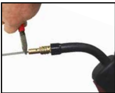
(7) Snip the liner off 3mm past the end of the torch neck.
