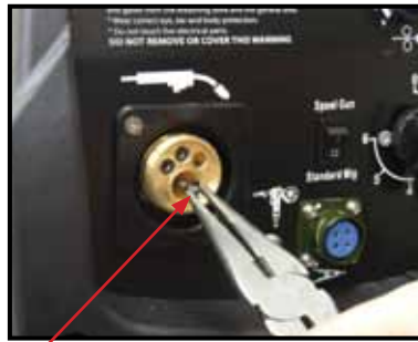
(11) Remove the inlet guide tube using long nose pliers.
