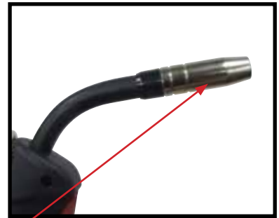
(14) Fit the gas nozzle to the torch head.
