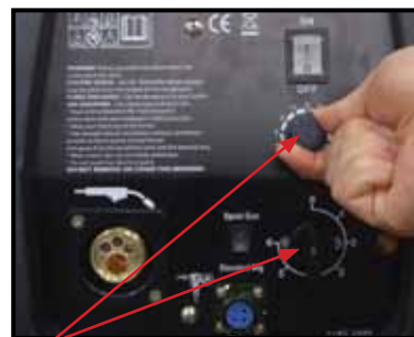
(17) Set welding parameters using the voltage and wire feed controls.
