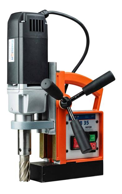
The Excision EMB35 magnetic based drill is the machine for the efficient drilling of holes under 35mm. Weighing only 10.6kg, this German made drill is durable for any small engineering application. The direct Weldon arbor type spindle is capable of handling all 19mm shank core drills.
